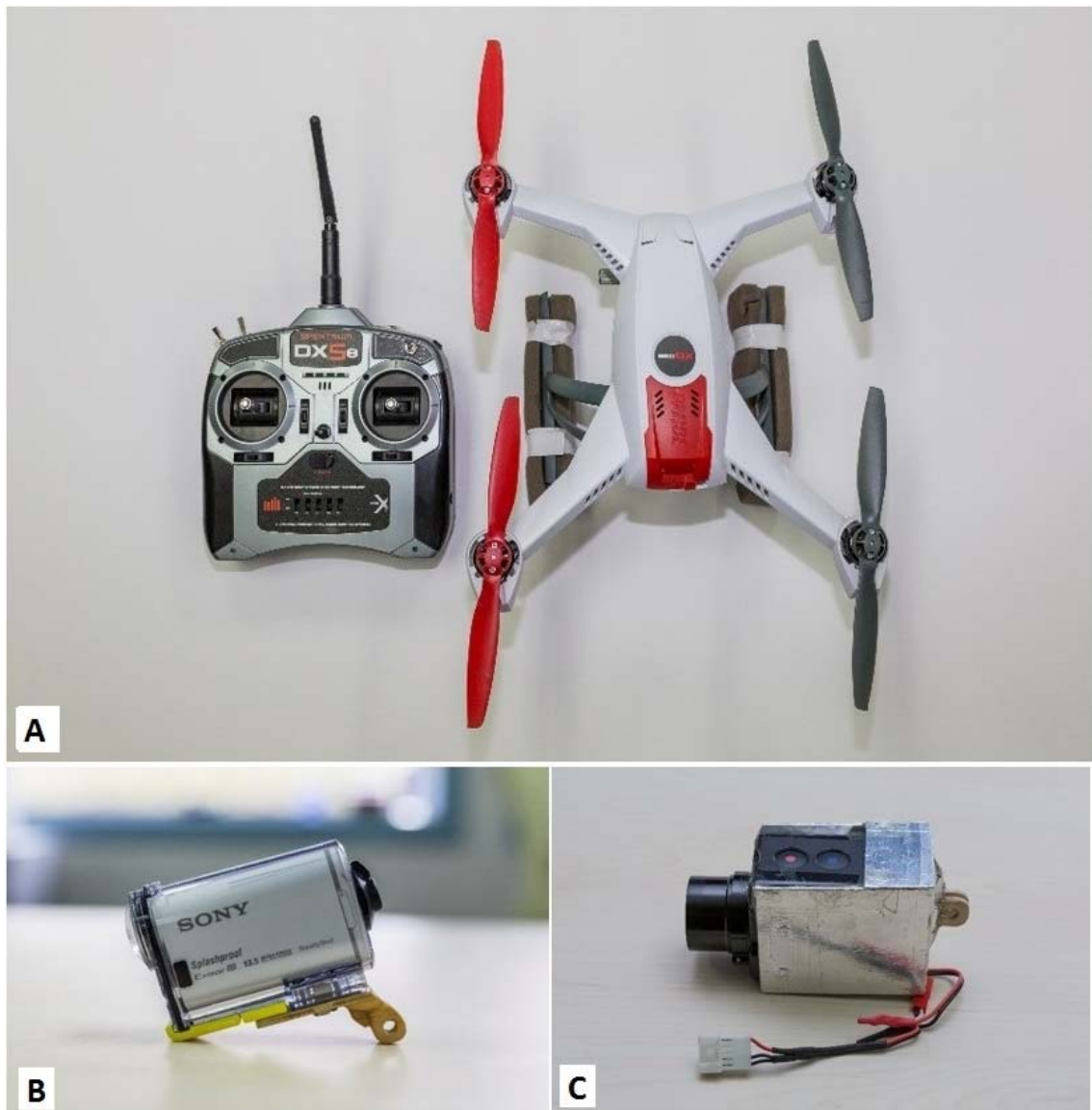
Figure 13. Drone and cameras used in this study. (a) Blade 350 QX2 Quadcopter with a Spektrum DX5e DSMX 5-Channel transmitter. (b) Sony HDR-AS100V action camera. (c) FLIR Tau 320 sensor covered with aluminium foil.
