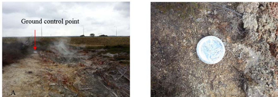
Figure 14. Picnic plates covered with aluminium foil used as ground control points.
