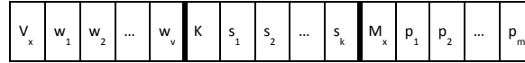
Fig. 6 A chromosome used in IMPM for the global optimisation of the parameters ('genes'): the variables V_x to be selected; their corresponding weights W_x ; number K of nearest neighbours to x_v ; the neighbourhood D_x with selected K samples s_1 - s_K ; a local prognostic model M_x (e.g. classifier); a parameter set P_m for the M_x .
