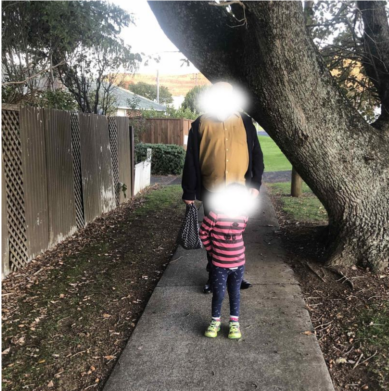
Figure 17: A tree trunk obstructing the footpath at head height and not detected by the long cane; photo contributed by Lenny
