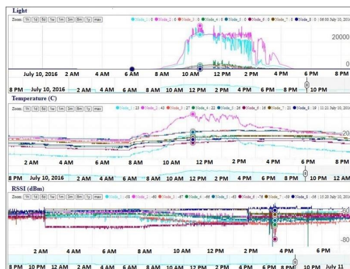
Figure 3-5 Graphical trend of sensor data (ambient light, temperature and RSSI) captured by the 8 leaf nodes, retrieved from Server database.
