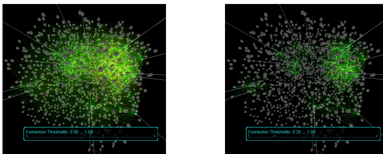
Fig. 6 Screenshots of NeuVis with the connection weight threshold set to show all connections (left) or only connections with a high weight (right), revealing connectivity clusters.
