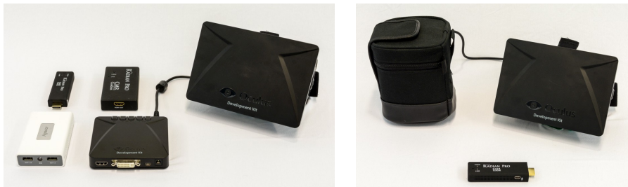
Fig. 11 Left: Components of the wireless HDMI transmitter system used for un-tethering users within the motion capture space (from left to right: Battery, transmitter, Oculus Rift breakout box, HDMI receiver). Right: Belt pouch containing all receiver and power components. The sender unit in front is connected to the stationary render computer.
