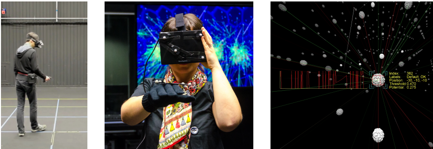
Fig. 5 User selecting a neuron via a 3D tracked joystick (left image) and a glove (centre image) to observe the activity of a specific neuron (right image).
