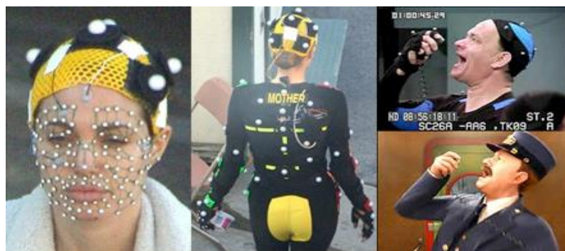
Figure 2: The passive markers in motion capture
