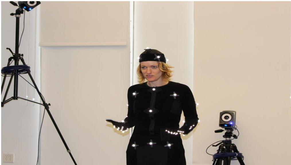
Figure 1 : The bright lights are actually lightweight reflectors
