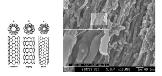
Fig. 2 Structure of carbon nano tubes.
