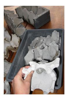
Fig 31 Moulds used to cast concrete. Resin impregnated plaster in background and in front flexible silicon version.
