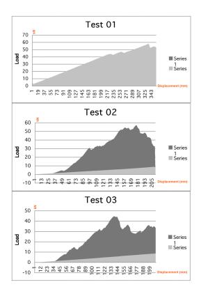
Graphs showing outcome of compressive tests with failure demonstrated at moment when the graph descends. Failure occurs at a load of 45, 56 and 42 kN.
