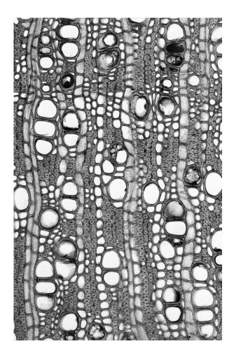
Fig. 3 Microscopic cross section of Olive wood showing variations in wall thicknesses, cell thicknesses and perforations.
