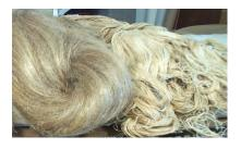
Fig. 19 Flax fibres left, have been used by the SHAC team from the Engineering School at Auckland University to reinforce a prototype or a sustainable thin walled composite panel system made with a matrix of 90% rammed earth and 10% concrete.
