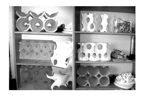
Fig. 26. Models testing scale of cells and mouldability with paper and plaster versions to right.  $\,$
