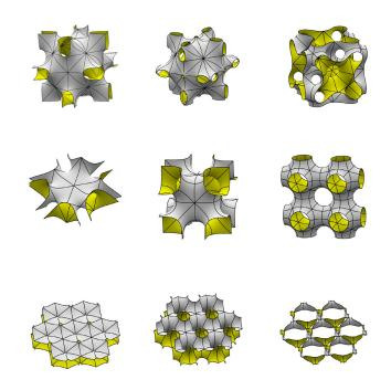
Fig. 21. Different types of minimal surface structures from left to right: Neovius' Surface, Neovius Complementary P surface, Schoen's Manta Surface of Genus 19, Schoen's Complementary D Surface, Schoen's I-WP Surface, Schwarz' P Surface, and variations of Schoen's Hybrid-I [P,F-RD] Surface.
