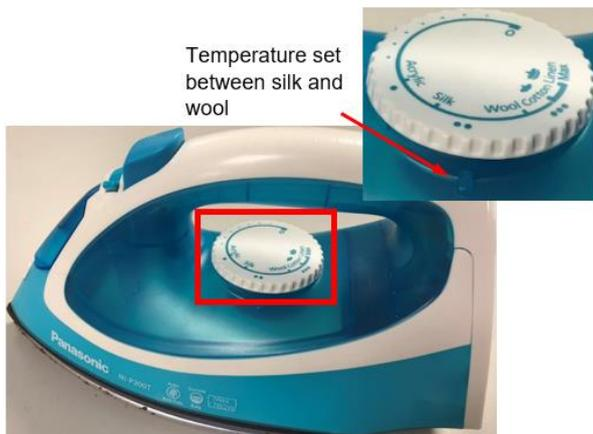
**Figure 5.1. Domestic steam iron (Philips NI-P300T) for bonding fabric materials.**
