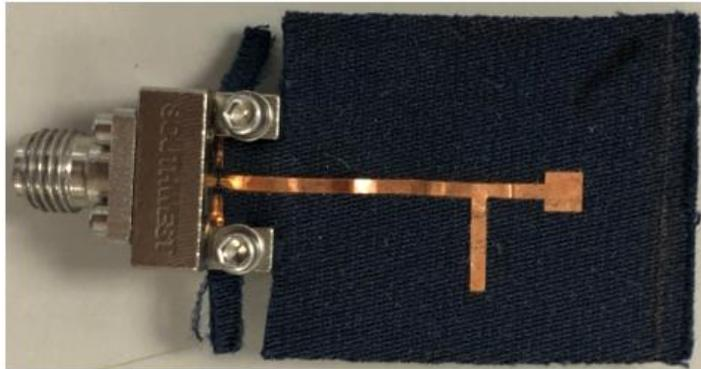
**Figure 6.9. Fabricated prototype of the humidity sensing antenna.**
