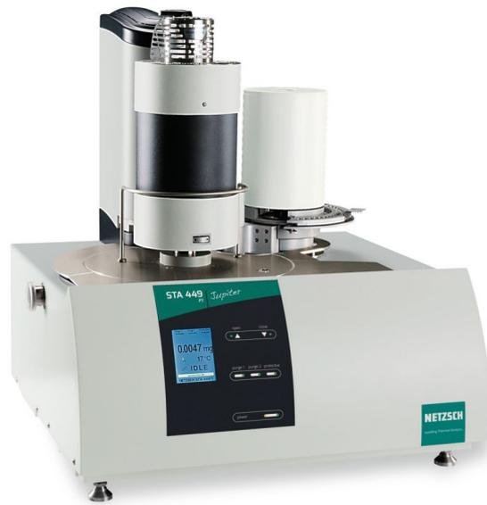
Figure 78. DSC Netzsch STA 449 F1 system
