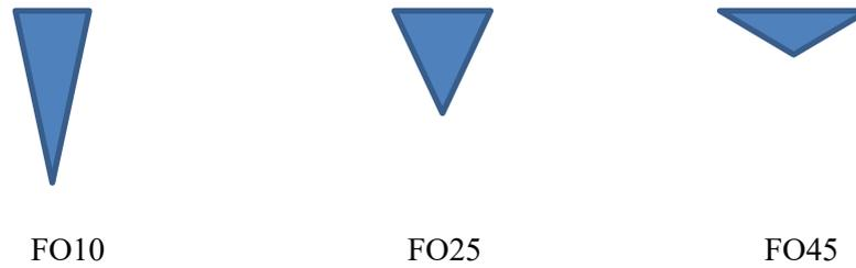
Figure 63. Melt pool geometries with different focus offset values
