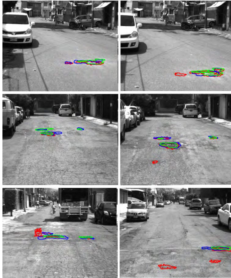
Figure 5.15: The potholes found using SV1 and SV2 approaches are marked in red and green respectively, while the manually labeled ground truths are marked in blue.
