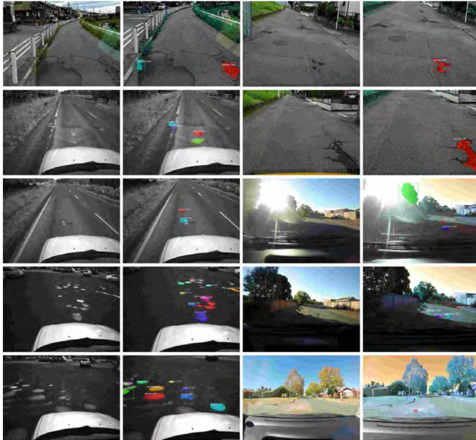
Figure 5.10: Detected “potholes” from the validation dataset using LM1, shown in two columns with original image on the left and predicted results on the right. Top to bottom, left to right. Ten frames in order as listed in Table 5.2.
