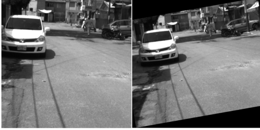
Figure 3.8: Original image on left side and transformed image on right side. The transformed image is resized at 0.7 times the original image and rotated at an angle of 10^\circ in the counterclockwise direction.
