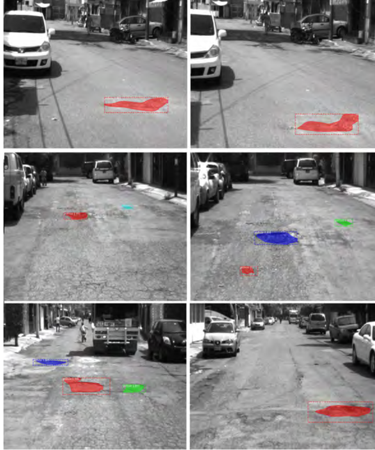
Figure 5.16: The potholes found using LM1 model and frames are same as Fig. 5.15.
