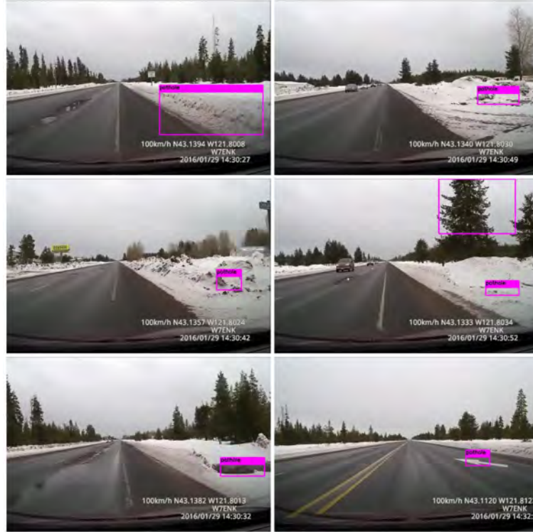
Figure 5.23: False detections identified using LM2 from PNW test dataset.
