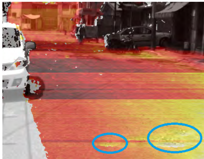
Figure 4.13: The brighter pixels indicate disparities that significantly smaller than the road manifold's disparities.
