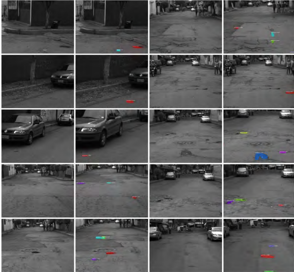
Figure 5.13: Detected road potholes of CCSAD Urban sequence 2 in upper figure LM1, with original image on the left and obtained results on the right. Top to bottom, left to right: Frames in order as listed in Table 5.2.
