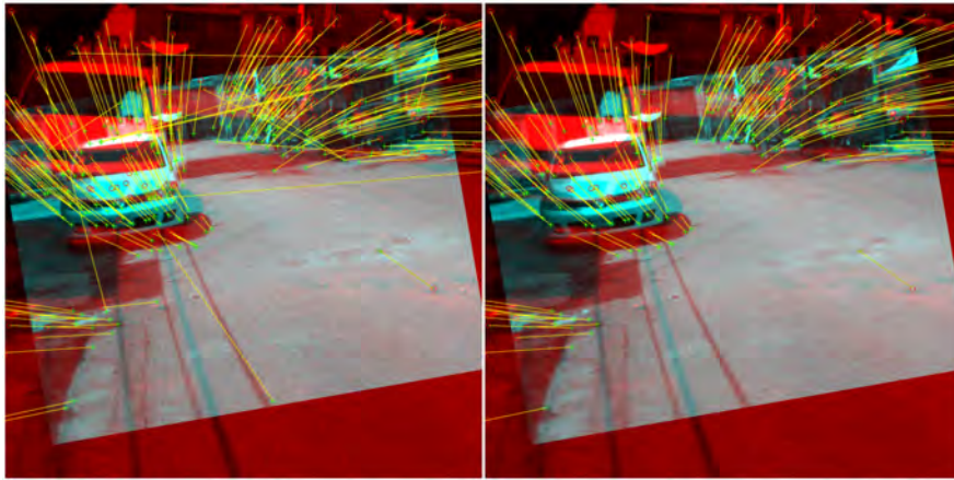
Figure 3.9: SURF keypoints matched on the left side including outliers. RANSAC for outliers removal for 1000 iterations on right side.
