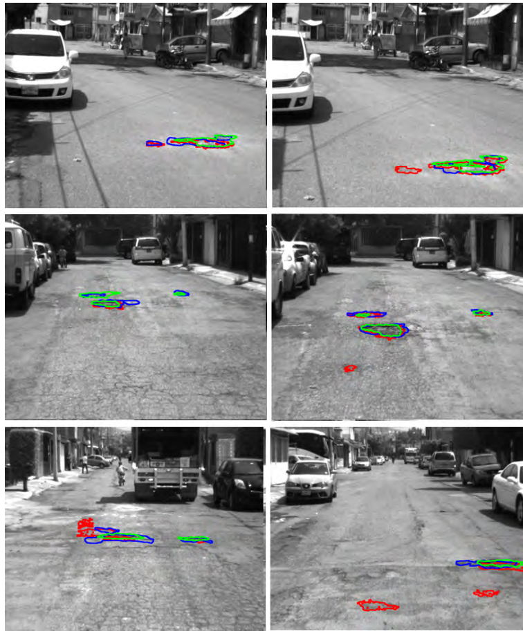
Figure 4.23: Tested frames and detected potholes. The potholes found using SV1 and SV2 approaches are marked in red and green respectively, while the manually labelled ground truths are marked in blue.
