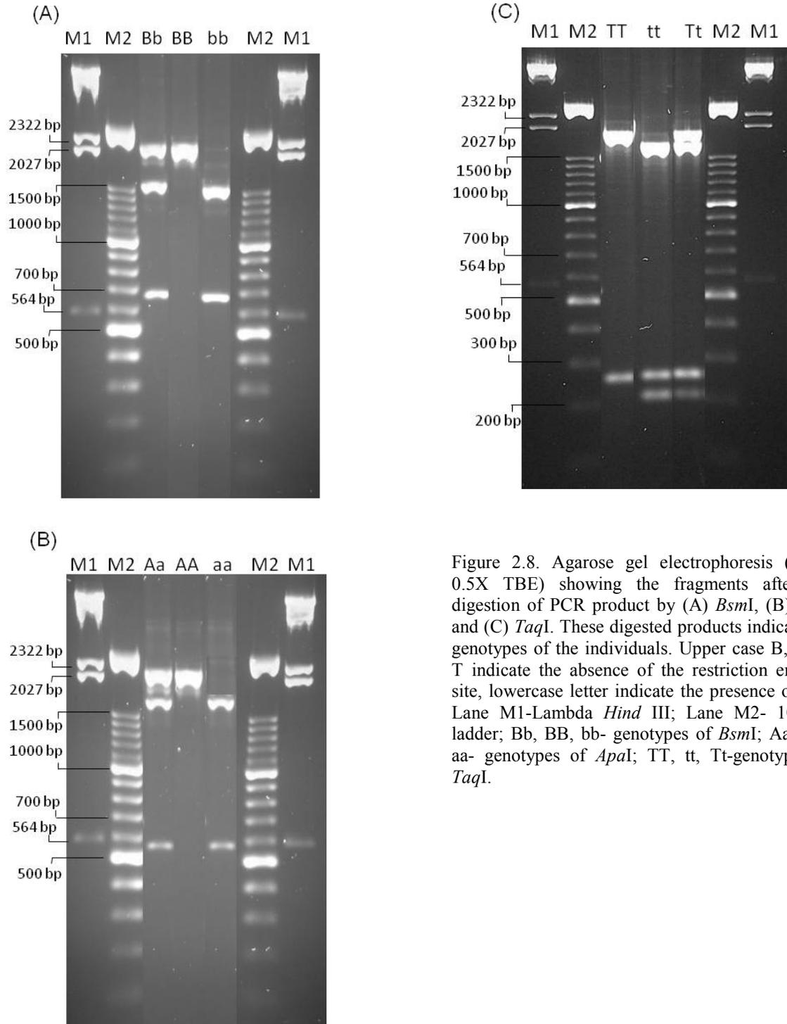
Figure 2.8. Agarose gel electrophoresis (1.4%, 0.5X TBE) showing the fragments after the digestion of PCR product by (A) *BsmI*, (B) *ApaI* and (C) *TaqI*. These digested products indicate the genotypes of the individuals. Upper case B, A, or T indicate the absence of the restriction enzyme site, lowercase letter indicate the presence of site. Lane M1-Lambda *Hind* III; Lane M2- 100 bp ladder; Bb, BB, bb- genotypes of *BsmI*; Aa, AA, aa- genotypes of *ApaI*; TT, tt, Tt-genotypes of *TaqI*.
