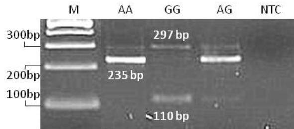
Figure 2.16. Gel electrophoretic separation pattern (2.5%, 0.5X TBE) of ASM-PCR of Cdx-2 products in 0.5X TBE buffer electrophoresed at 120V and visualised after 1 hour. AA, GG and AG-genotypes of Cdx-2 SNP; Lane NTC-no template control.
