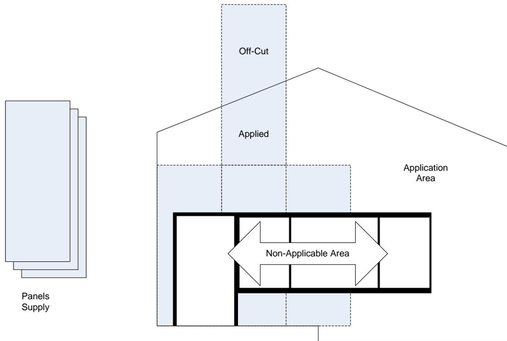
**Figure 3.1: Wall Overlay with Fixed Size Panels**
