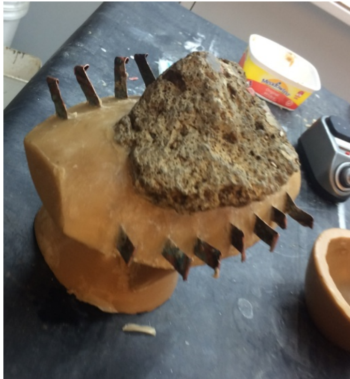
Fig.2.14. The end of the first stage of casting. Here is the finished wax object ready for the next stage.
