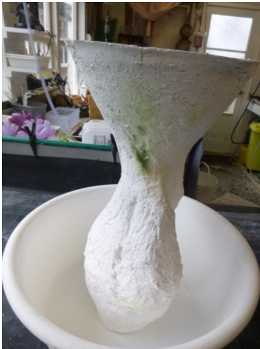
Fig. 3.05. This is an object just cooled and is ready to be divested. Of note are the interesting green marks on the mould surface.
