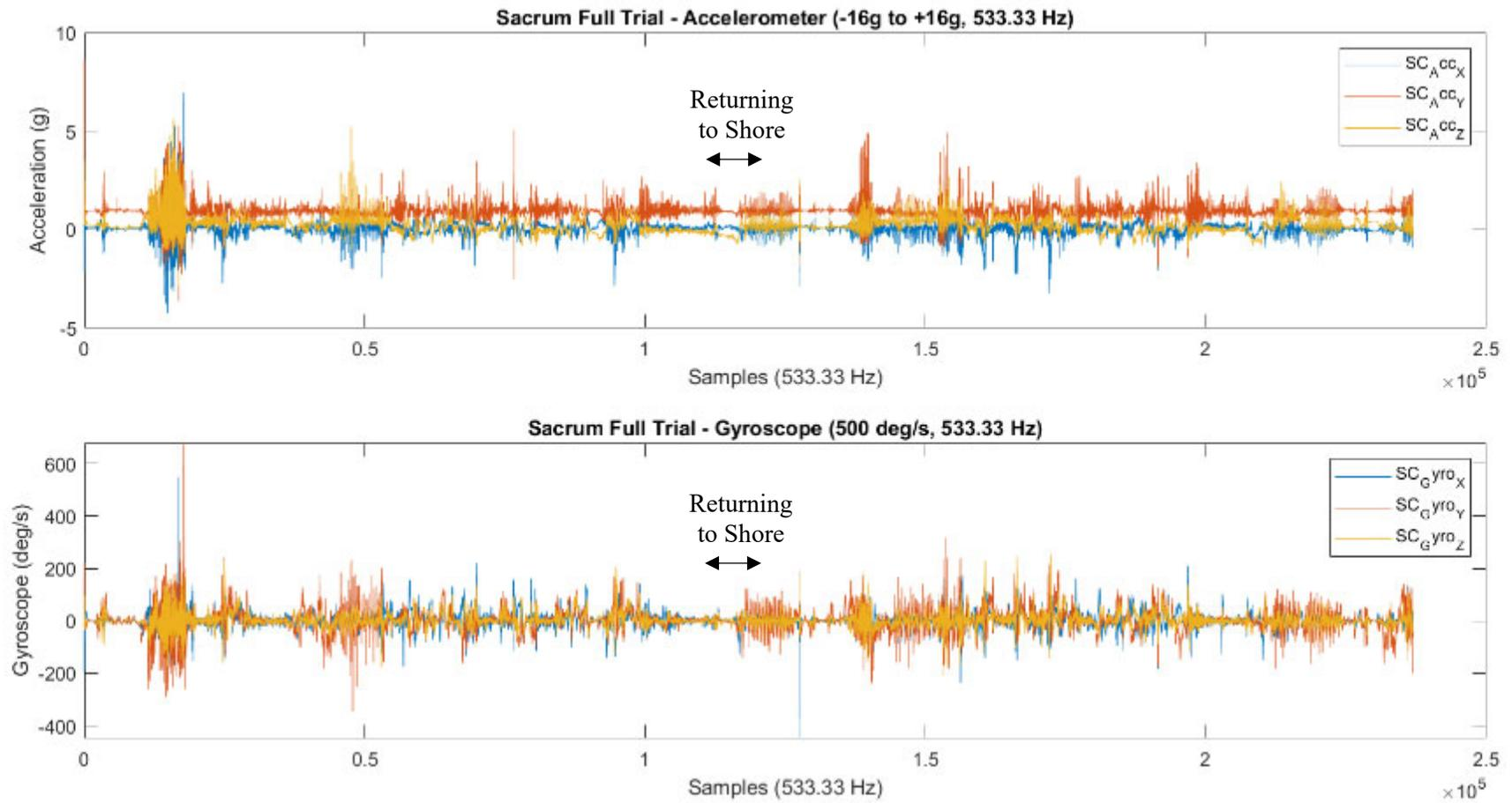
Figure 13: Sacrum - Full Trial Accelerometer and Gyroscope Raw Data (7:23)
