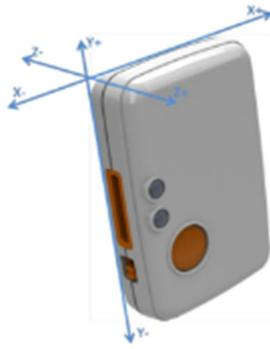
Figure 8: Shimmer3 IMU orientation.
