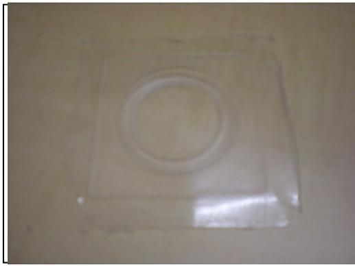
**Figure 4. 11: Corrugated PDMS diaphragm**
