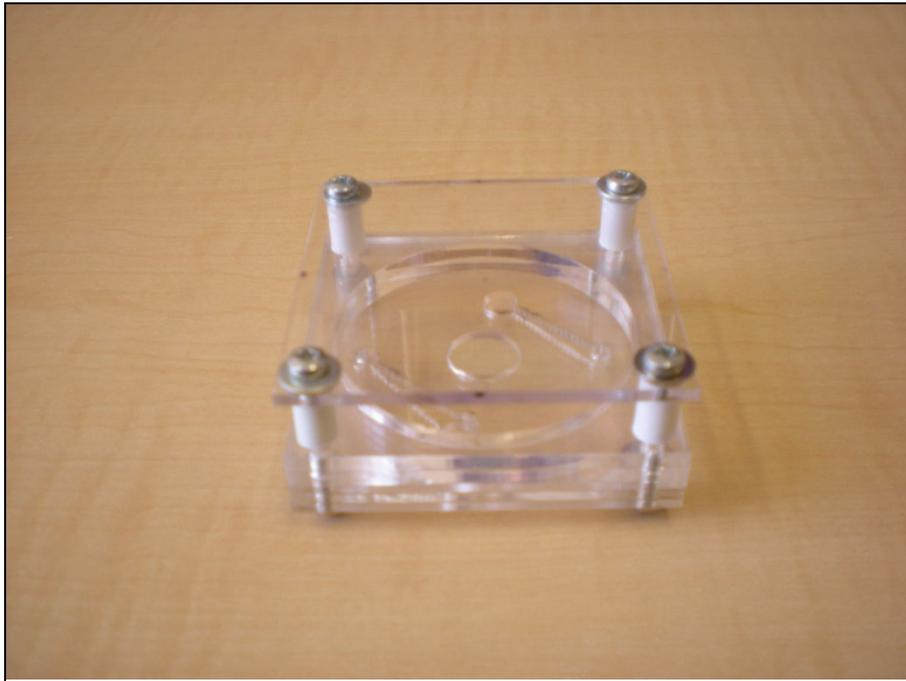
**Figure 4. 15: Chamber with nozzle/diffuser under it**
