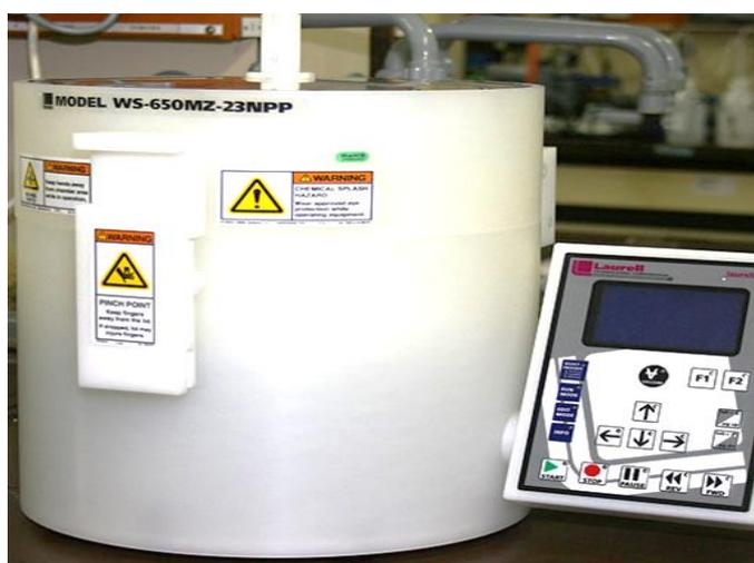
Figure 4.3 Spin coater used for Microfabrication
