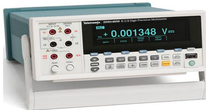
Figure 3.9 Digital Multimeter to measure the in-plane resistance
