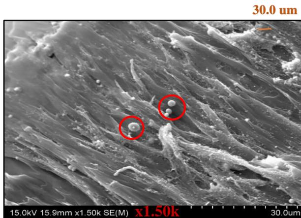
Figure 5.16 Balling effect in SEM image for 95% PA/5% Ti-Nano
