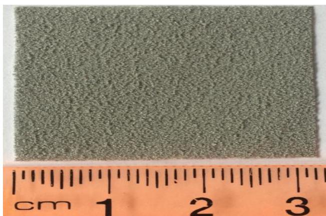
Figure 4.2 Actual Photograph of Alumide Thin film
