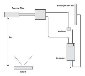
Figure 2: Arrangement of Devices
