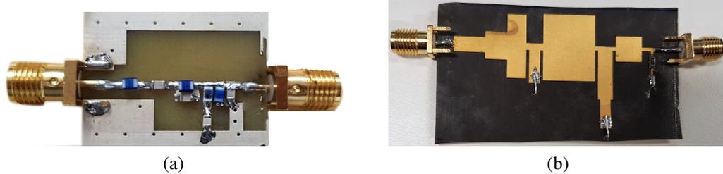
Figure 3.12: Fabricated DBIMN Prototype (a) with lumped elements (b) microstrip distributed elements
