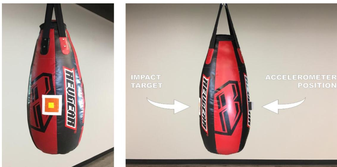
**Figure 8.** A front and side view of a similar tear drop bag equipped with an accelerometer and marked with an impact target.
