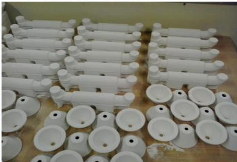
**Fig 2.8. Printed Moulds and pouring cups waiting to be cast**
