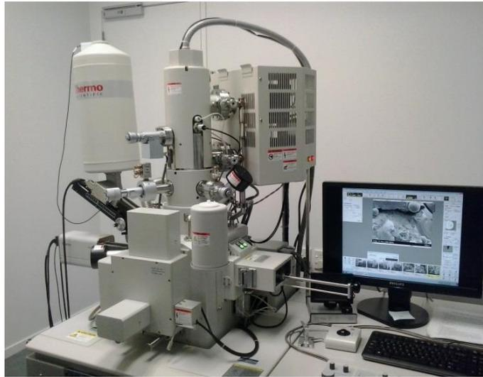
***Fig2.3. The Hitachi SU-70 Schottky field emission SEM***
