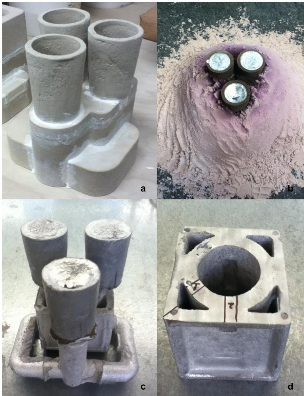
**Fig. 6.16** The casting process and outcomes (a) assembled mould, (b) aluminium filled in the mould backed-up by foundry sand, (c) the solidified shape, and (d) final casting
