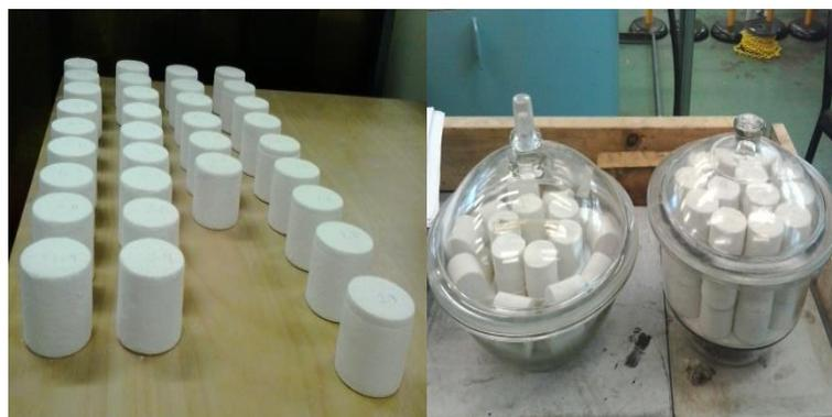
**Fig 2.5. Test specimens printed for compression tests as per the ASTM standards and preserved in the desiccator**
