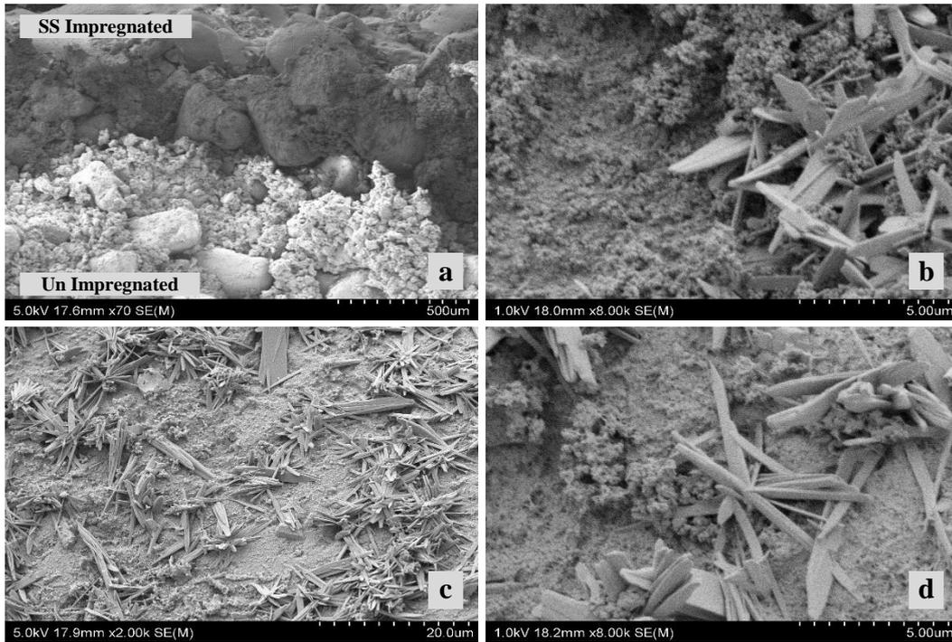
**Fig A2.20(a) Sodium silicate impregnated and un-impregnated zones of the baked mould wall, (b) Crystals of  $\alpha$ -HH and sodium silicate at impregnated zone,(c & d) Crystals of  $\alpha$ -HH at un-impregnated zone.**
