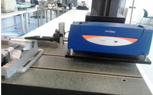
**Fig 2.12. The Taylor Hobson Talysurf surface roughness tester**
