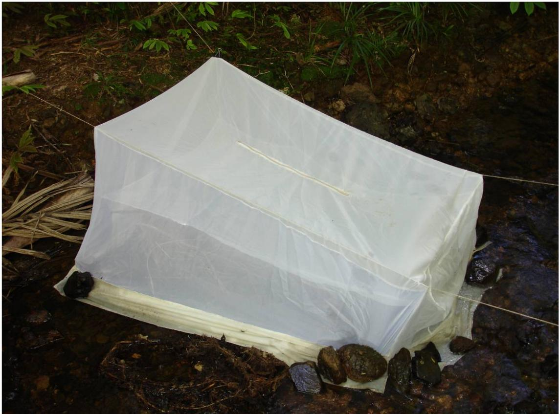
**Figure 34.** Final emergence trap design erected in the field. Access to the catch is through the central zip on the top, and the false collection base is clearly visible half-way up the inside of the trap.
