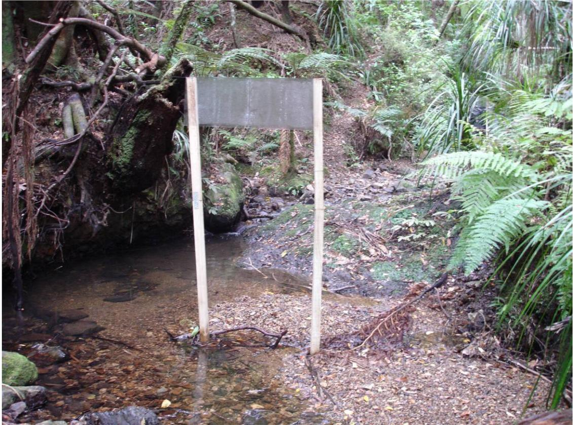
**Figure 21.** An improved version of the sticky trap system set in the field.
