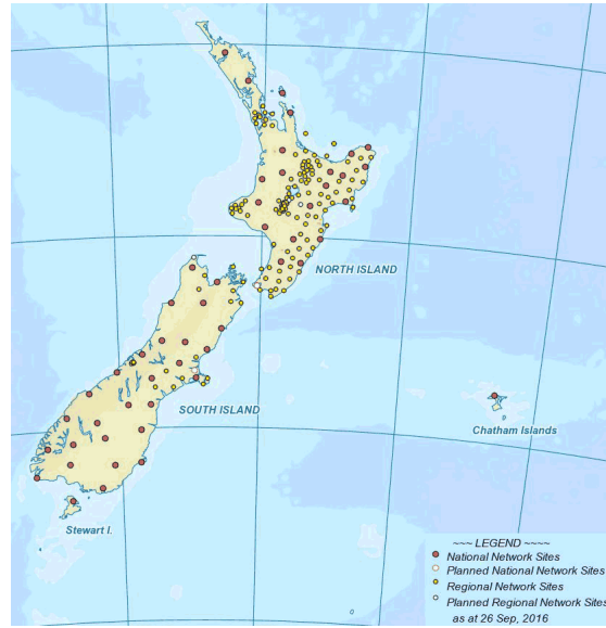
Figure 6.3: The New Zealand National Seismograph Network consists of primary sites located at approximately 100 km spacing, with extra regional sites established at places of geophysical significance.
