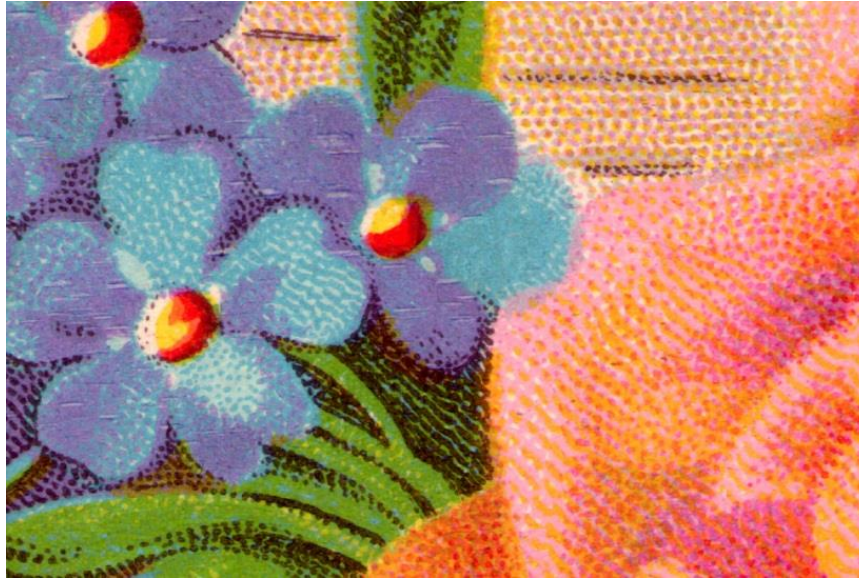
Figure 44: Detail showing the chromolithographic process Chromolithography involved the layering of multiple colours, each printed on a different stone. High quality cards routinely used between eight and twelve stones. The process typically uses a blend of flat colour and stippling. This image is from a 1913 German-printed postcard, but the technique is little changed from the earliest cards. Author's collection
