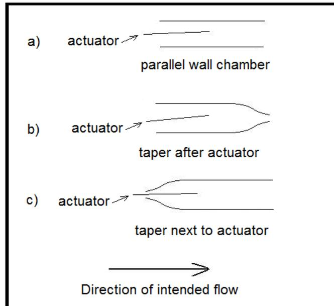
**Fig. 3.6** Three different actuator enclosure designs for the same air flow direction
