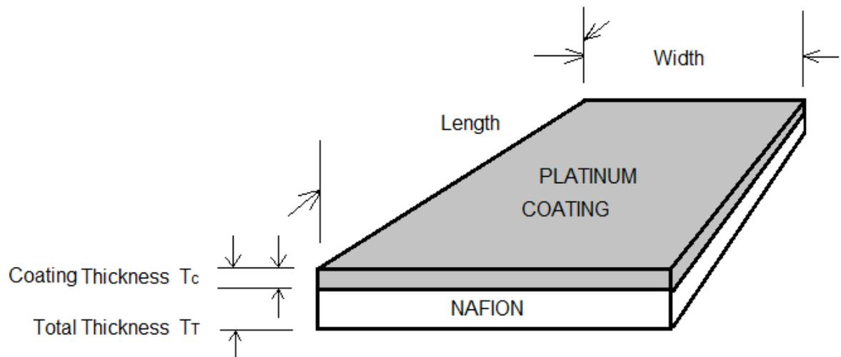
**Fig. 3.4** Geometry of coating thickness calculation assumptions
