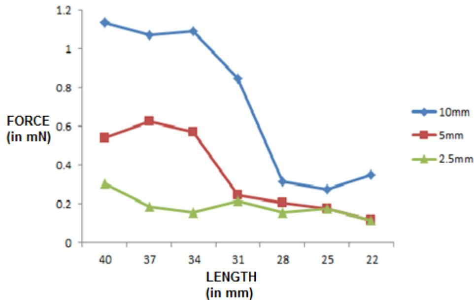
**Fig 4.5** Force of IPMC against Length at constant Voltage for three sample widths
