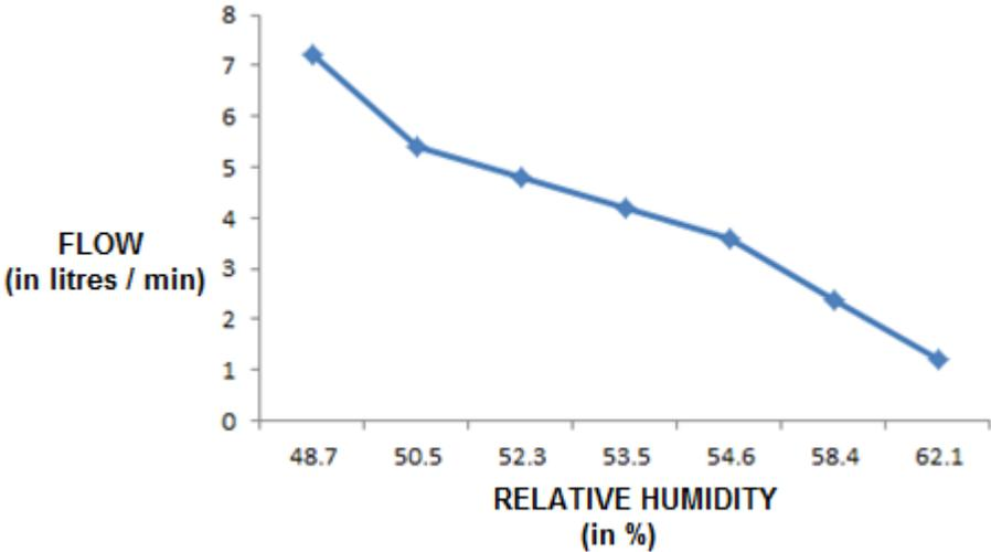
**Fig. 4.12** Flow rate versus relative humidity at 135mm depth H2O immersion
