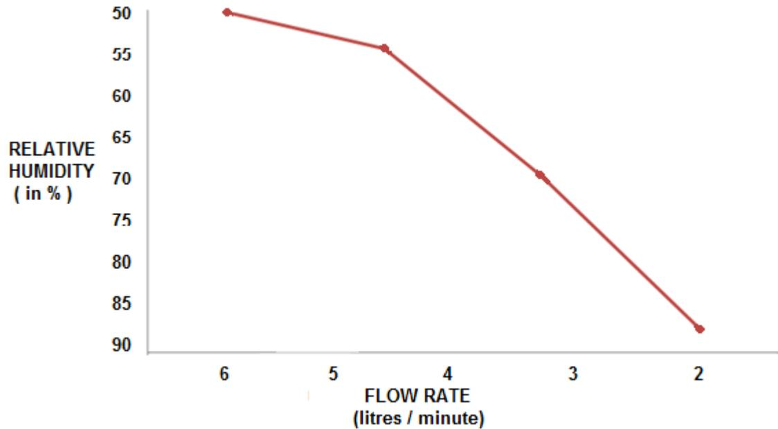
**Fig. 4.11** Relative Humidity of Exit Air versus Flow Rate
