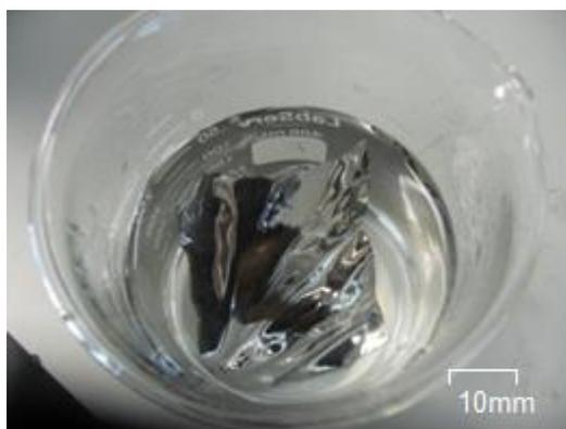
**Fig. 3.2** Smooth surface appearance of Nafion being platinum coated in solution
