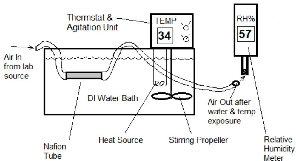
**Fig. 3.11** Temperature control humidification apparatus
