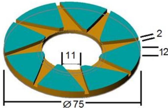
**Fig. 4.14** Theoretical eight chamber inward flowing spiral stack design
