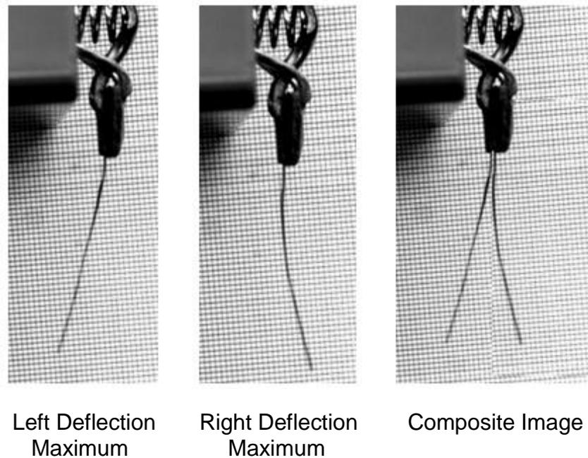
**Fig. 4.7** Video of Maximum Left and Right Pt-Nafion deflections and compound image of both
