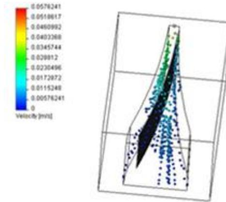
**Fig 4.8** Air flow speed CFD 2D model output
