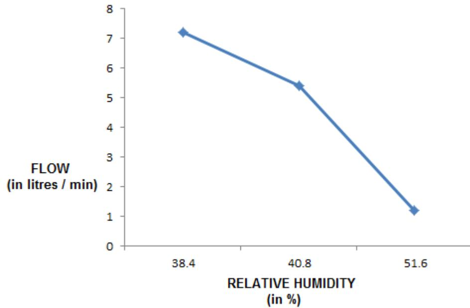
**Fig. 4.13** Flow rate versus Relative Humidity at 10mm depth H<sub>2</sub>O immersion
