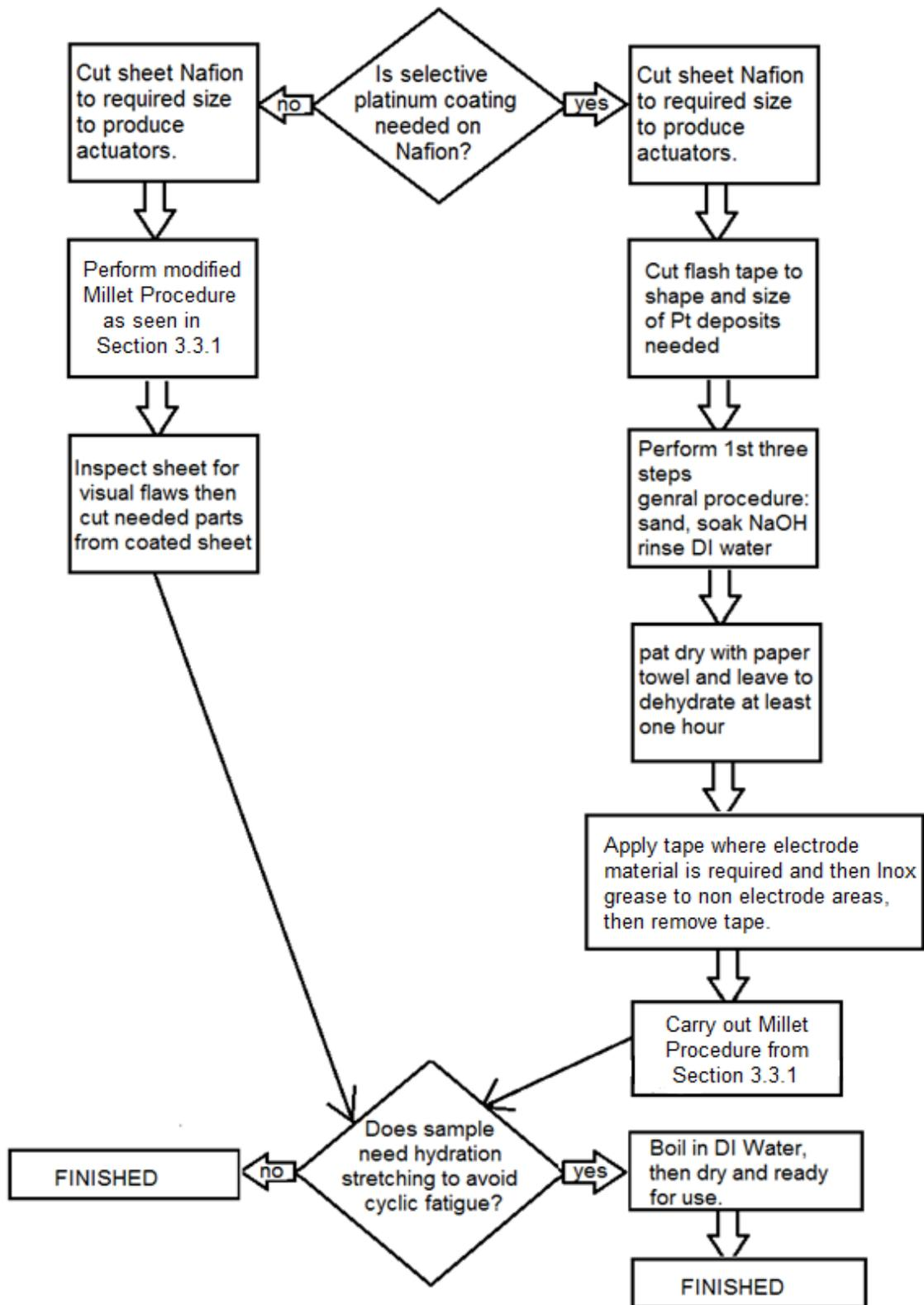
**Fig. 3.1** Coating Process Flow Chart
