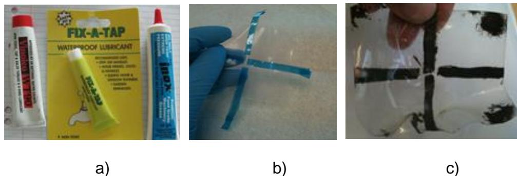
**Fig. 3.3** a) Grease options to test b) tape masking c) resulting Pt electrodes on sheet Nafion
