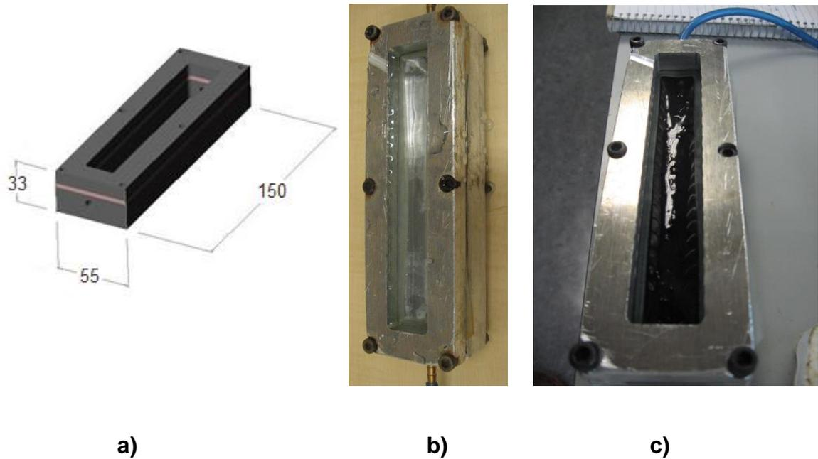
**Fig. 3.13** Trench fixture a) Design Nafion sheet b) untreated and c) treated sheet
