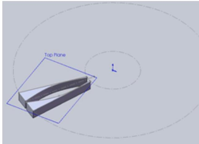
**Fig. 4.15** An enclosure shape that decreases the output area, but mimics the oscillation shape might increase flow speed
