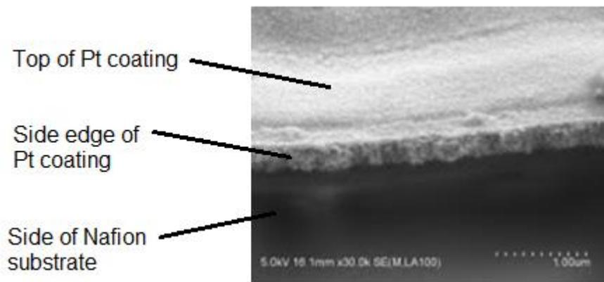
**Fig. 4.3** Thickness of Platinum coating on Nafion Substrate shown in SEM image
