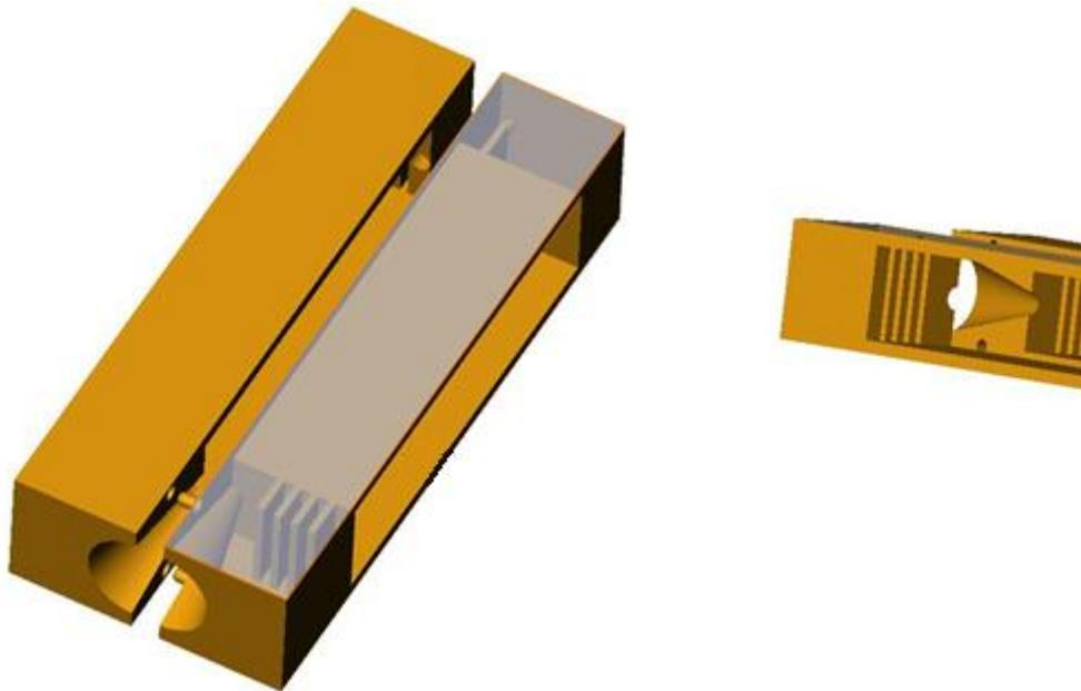
**Fig. 3.8** Diffuser modeled after actuator enclosure to investigate flow
