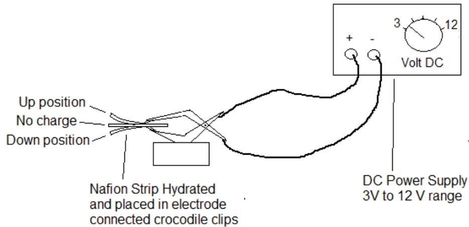
**Fig. 3.5** Actuation apparatus for first actuation testing
